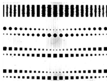
Figure 22 - Worst Stencil for Bottom Side Paste Smear
